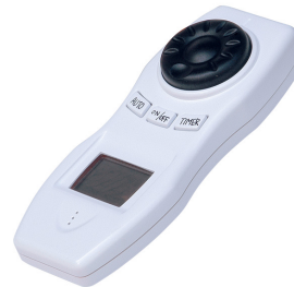
Hand control module with speed dial, timer and manual / auto mode buttons, and LED screen
